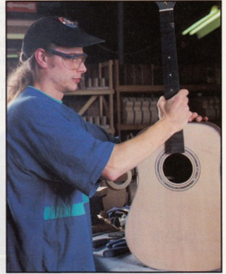
Fitting the neck to a Dreadnought body at the Guild factory in Westerly, Rhode Island.
